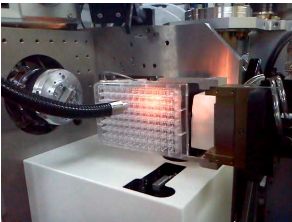
Figure 4. BL13-XALOC: A 96-well Greiner crystallization plate being scanned with the automated sample changer (robot) during the site acceptance tests.
